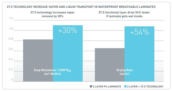
MORE THAN JUST MVT: The AATCC 201 test method begins to measure the movement of moisture at very low humidity levels using real life sweating rates. All other MVT tests are conducted using extreme sweating rates at humidity levels where you are already uncomfortable.
