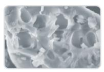
The desiccant nature of highly porous 37.5 active particles attracts moisture vapor. These particles release the water vapor by capturing your IR energy. This reoccurring capture and release mechanism pumps water vapor out of the garment system, enhancing the user experience. An 800% increase in surface area improves fabric drying times by 30 to 100%.
